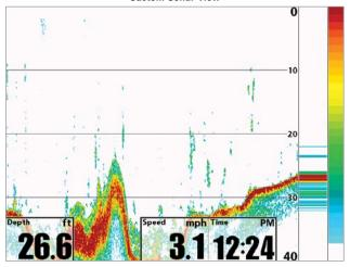
**NOTE:** When the readout under the water column is turned off (as shown in the illustrations), the sonar display will expand to fill the screen.
